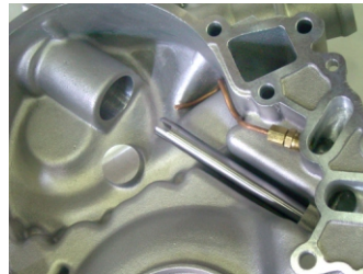
Distributor Gear Oiler
